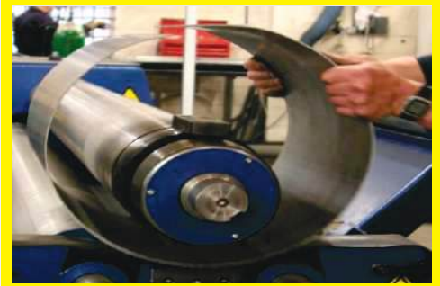
ROLLING AND BENDING (EVEN 500 BHN PLATES.)
